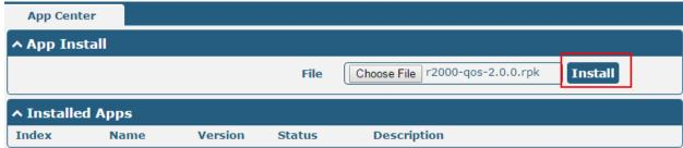
When the rate of installation progress reach 100%, the system will pop up a reboot router reminder window. Please click "OK" to make router reboot.
