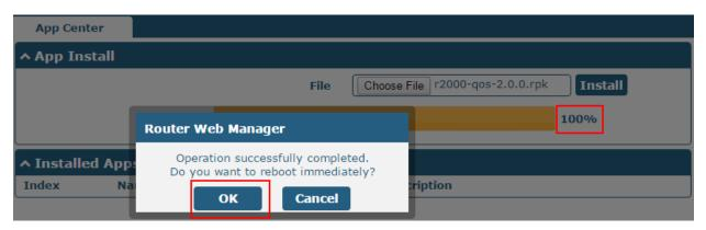
4 After router power on again, log in configuration page, QoS will be include in App Center's "Installed Apps" list, and the function configuration will display in **Network** part.
