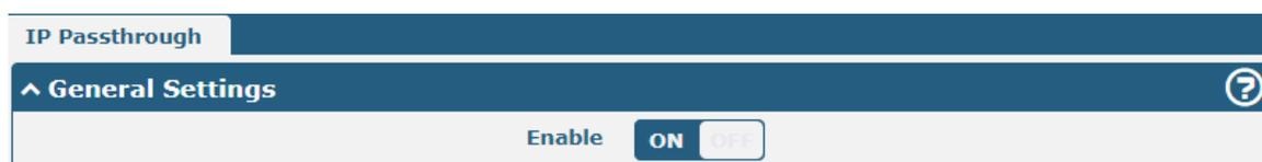
When gateway open IP Passthrough function, the end device (e.g.: PC) will open DHCP Client mode and connect to LAN port. After gateway dial successfully, PC will automatic obtain IP address and DNS server address assigned by the carrier.
