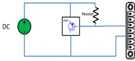
DO connect to PNP transistor(OUT1 for example)
