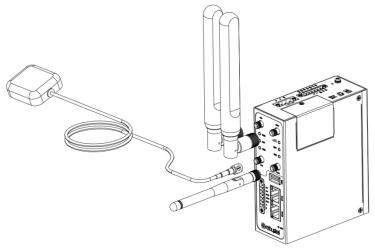
**3. Terminal Block Installation.** Insert the terminal blocks into the interfaces connector, then can connect the devices or sensors to the gateway via corresponding interfaces e.g. RS232/RS485, DIDO...
