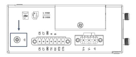
**6. Power Supply installation.** Following to the color of the head, connect the cable marked red to the positive pole through a terminal block, and connect the yellow one to the negative in the same way. The last step is to plug the power adapter into your socket.
