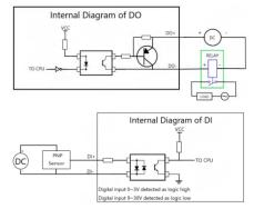
Note: The external power supply DC voltage range is 5V~30V, 0.1A max.
