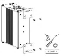
Grounding the Device. Grounding will help to prevent the noise effect due to electromagnetic interference (EMI). Connect the device to the site ground wire by the grounding screw before powering on.
