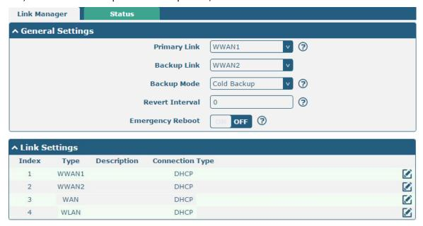
Click the <a> button of WWAN1 to set its parameters according to the current ISP.</a>
