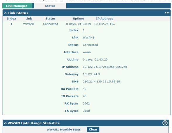
Click the **Clear** button to clear SIM1 monthly data traffic usage statistics. Data statistics will be displayed only if enable the Data Allowance function in **Interface > Link Manager > Link Settings > WWAN Settings > Data Allowance**.
