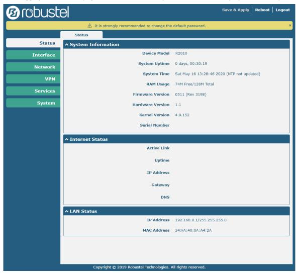
From the homepage, users can perform operations such as saving the configuration, restarting the gateway, and logging out.
