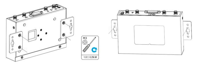
Use 4 pcs of M3 screws to fix the wall mounting kit to the gateway, and then use 2 pcs of M3 drywall screws to mount the gateway associated with the wall mounting kit on the wall.
