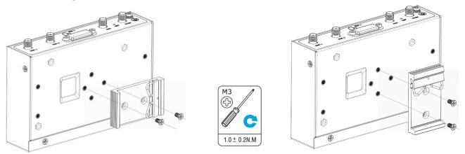
Use 3 pcs of M3 screws to fix the DIN rail to the gateway (as illustrations above shown, there are two mounting angles to choose from), and then hang the DIN rail on the mounting bracket.
