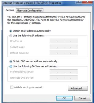
Manually configure the PC with a static IP address on the same subnet as the gateway address, click and configure "Use the following IP address";
