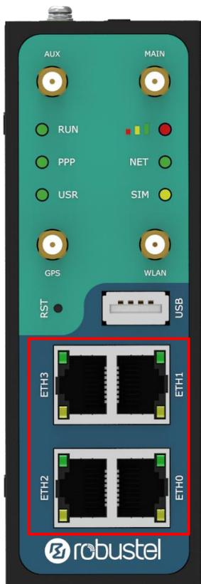
R3000 Quad Router has four Ethernet port with two LED indicators. The yellow one is link indicator and the green one is speed indicator. For details about status, see the table below.
