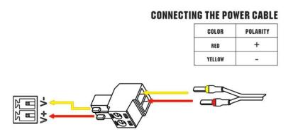
R1511 Router doesn't support reverse polarity protection; always refer to the figure above to connect the power adapter correctly. There are two cables associated with the power adapter. Following to the color of the head, connect the cable marked red to the positive pole through a terminal block, and connect the yellow one to the negative in the same way.
