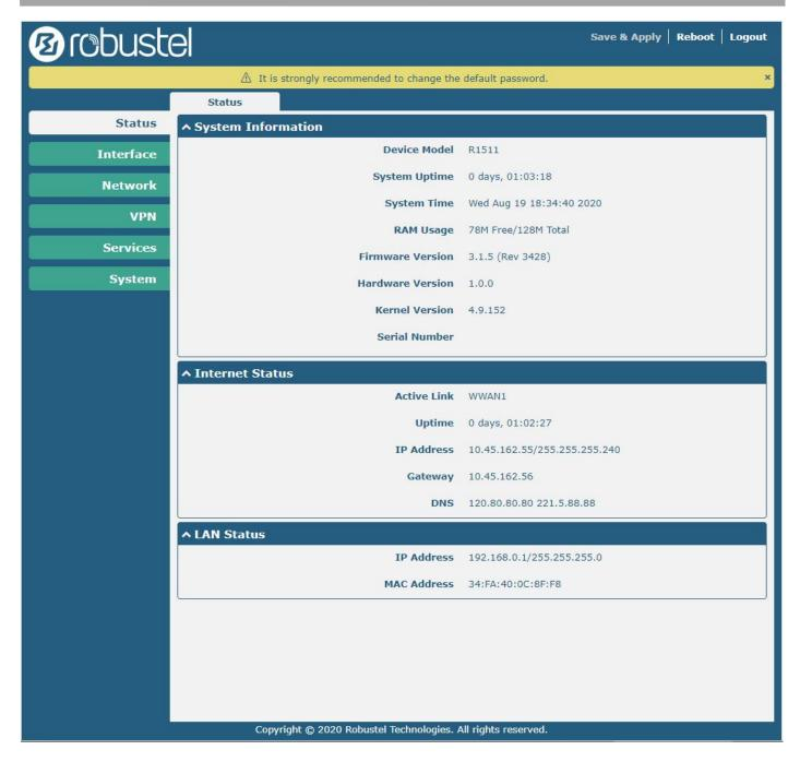
In the home page, the user can save the configuration, restart the router, log out, and so on. Using the original username and password to log in the router, the page will pop up the following tab.
