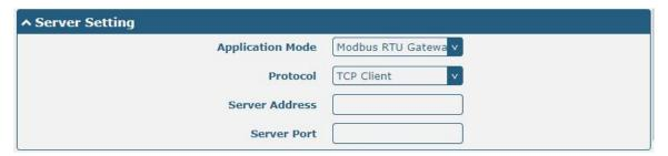
When selecting "ModBus RTU Gateway" as the application mode and "TCP Server" as the protocol, the window is as
