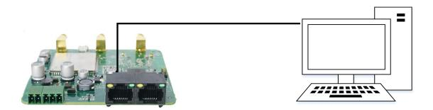
Connect a standard Ethernet cable to the port marked ETH0~ETH1 at the front of the R1511P Router, and connect the other end of the cable to your computer.
