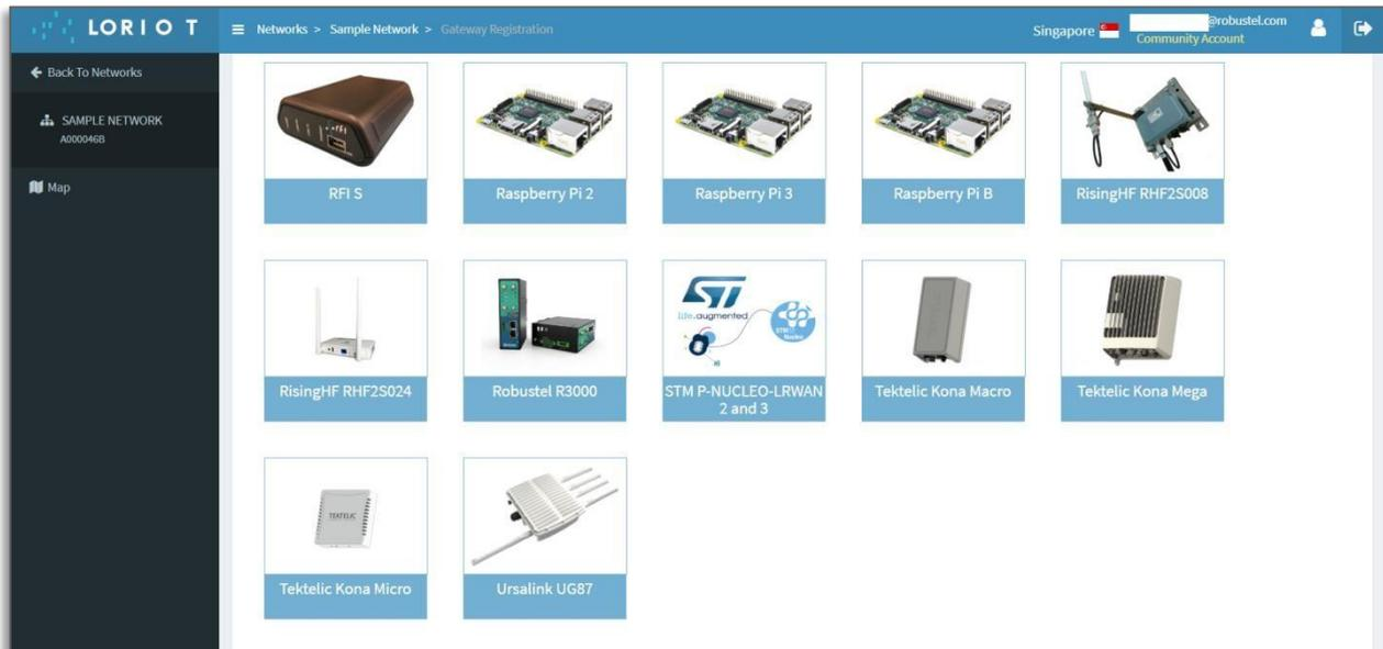
Figure 2.5 – Select the R3000 LG from LORIOT Gateway menu scree
