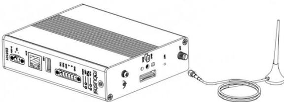
3. **Terminal Block Installation.** Insert the 6PIN terminal block into the interfaces connector, then can connect the devices or sensors to the gateway with wires via corresponding interfaces e.g. RS232/RS485
