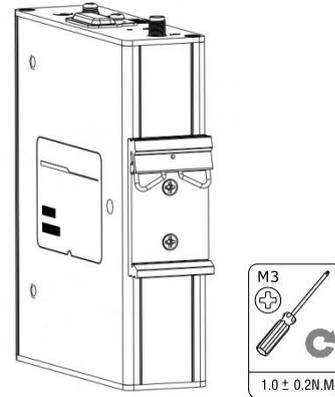
6. **Wall Mounting.** Use 2 M3 screws to fix the Wall mounting to the device.
