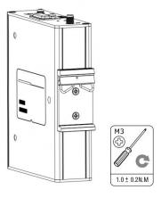
**6. Wall Mounting.** Use 2 M3 screws to fix the Wall mounting to the device.
