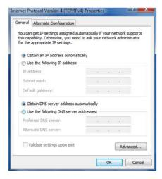
Use the following IP address (configured a static IP address manually within the same subnet of R2000 Dual Router):
