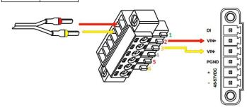
**Step 7:** R2000 Dual Router also supports POE feature. Please refer to the figure below to connect the power adapter correctly.
