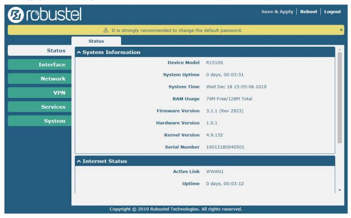
In the home page, the user can save the configuration, restart the router, log out, and so on.
