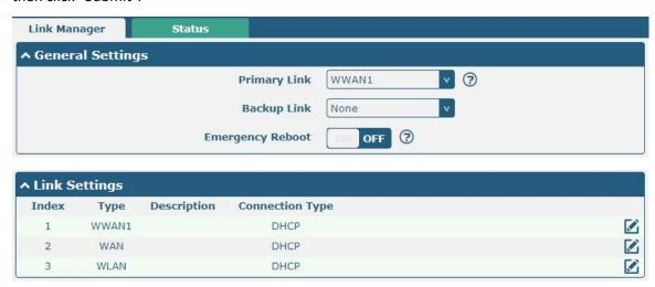
Click the right most of edit button of WWAN1 to set its parameters according to the current ISP.
