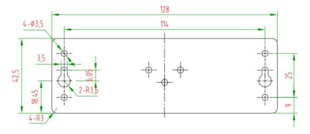
Use 3 pcs of M3 screws to mount the router on the wall mounting kit, and then use 2 pcs of M3 screws to mount the wall mounting kit on the wall.
