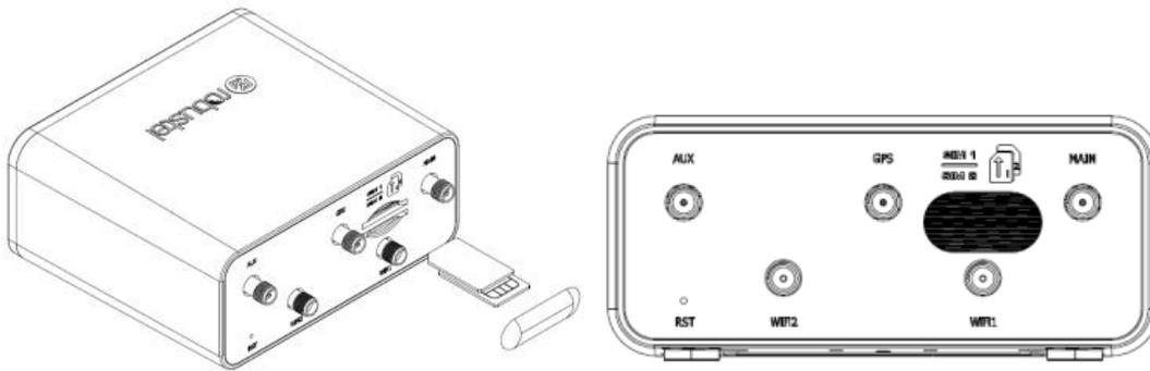
2. **Antenna Installation.** Rotate the antenna into the antenna connector accordingly.
