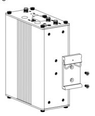
5. Grounding the Device. Grounding will help to prevent the noise effect due to electromagnetic interference (EMI). Connect the device to the site ground wire by the grounding screw before powering on.
