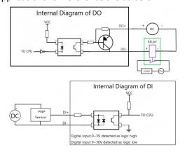
Note: The external power supply DC voltage range is 5V $^{\sim}$ 30V, 0.1A max.
