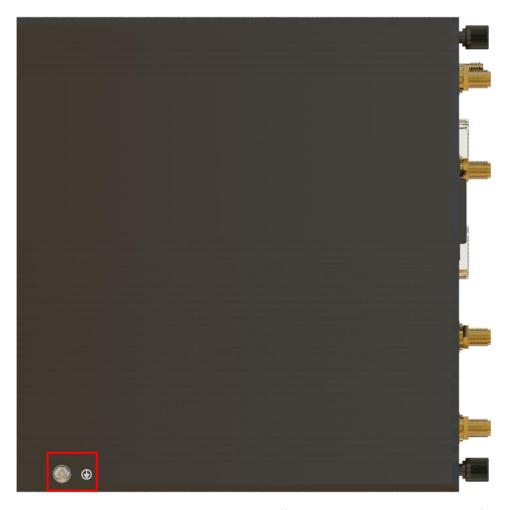
Gateway grounding helps prevent the noise effect due to electromagnetic interference (EMI). Connect the gateway to the site ground wire by the ground screw before powering on.
