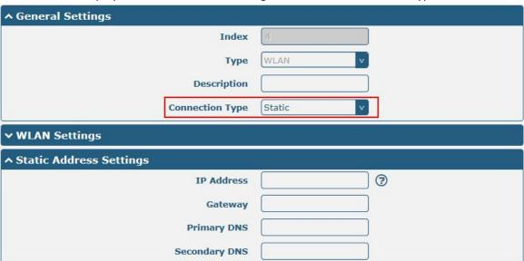
MEG5000 does not support the **PPPoE** WLAN Connection Type.
