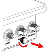
2. Connect a power supply cable to the power port, and rotate it clockwise.
