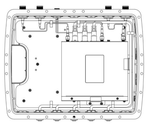
2. Disconnect all cables or wires of the router and take it out.
