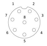
When the serial port is RS485+RS485, the pins are defined as follows:
