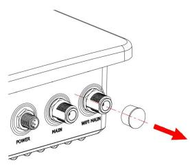
2. Connect the antenna to the corresponding antenna connector by holding onto the metal part of the antenna and rotating it clockwise. **Note**: Each antenna is labeled as 3G, 4G or WiFi for easy installation.
