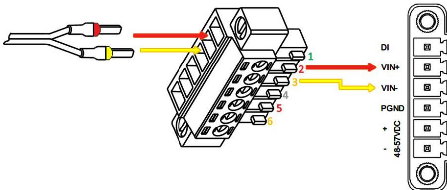
R2000 Dual Router also supports POE feature. Please refer to the figure below to connect the power adapter
