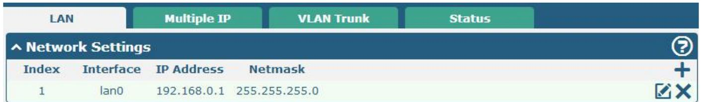
Click to edit the configuration of the current LAN interface. Click to delete the current LAN interface. Click to add a new LAN interface. The maximum number of LAN interface is four which include lan0, lan1, lan2 and lan3.
