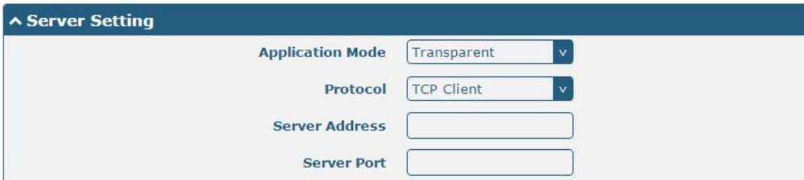
The screenshot shows a 'Server Setting' window with a blue header. It contains four fields: 'Application Mode' is a dropdown menu set to 'Transparent'; 'Protocol' is a dropdown menu set to 'TCP Client'; 'Server Address' is an empty text input field; and 'Server Port' is an empty text input field.
