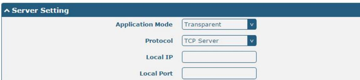
The screenshot shows a 'Server Setting' window with a blue header. It contains four fields: 'Application Mode' is a dropdown menu set to 'Transparent'; 'Protocol' is a dropdown menu set to 'TCP Server'; 'Local IP' is an empty text input field; and 'Local Port' is an empty text input field.
