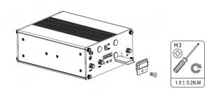
Antenna Installation. Rotate the antenna into the antenna connector accordingly.
